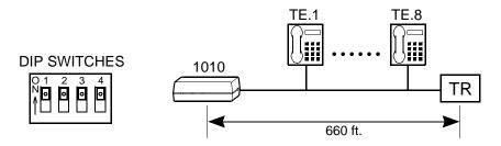
Figure 9—Extended Passive Bus (Cluster Multipoint)
